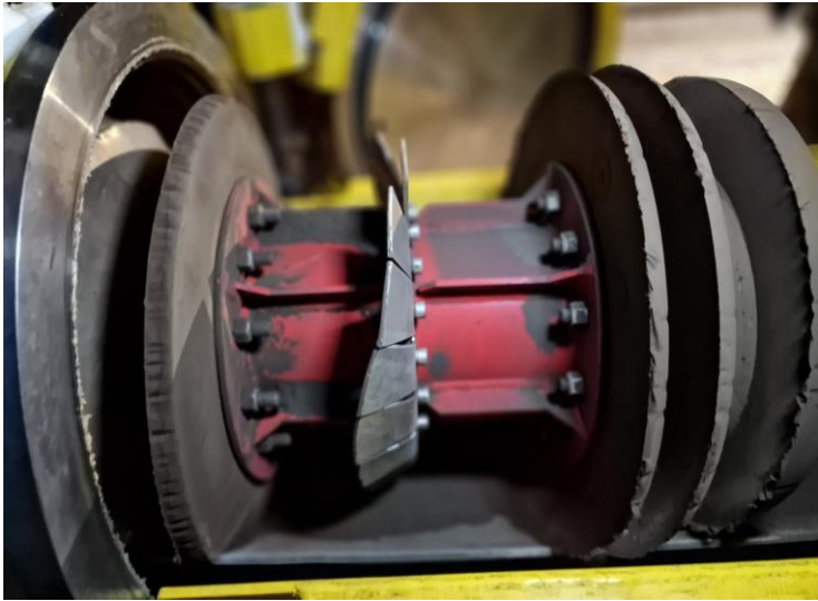
Pictures of cleaning tool with calibration plate
