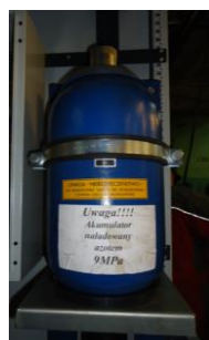
→ Hydraulic Accumulator for Emergency Fast Operations
