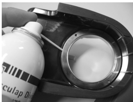
Fig. 24: Lubricating the lens holder
