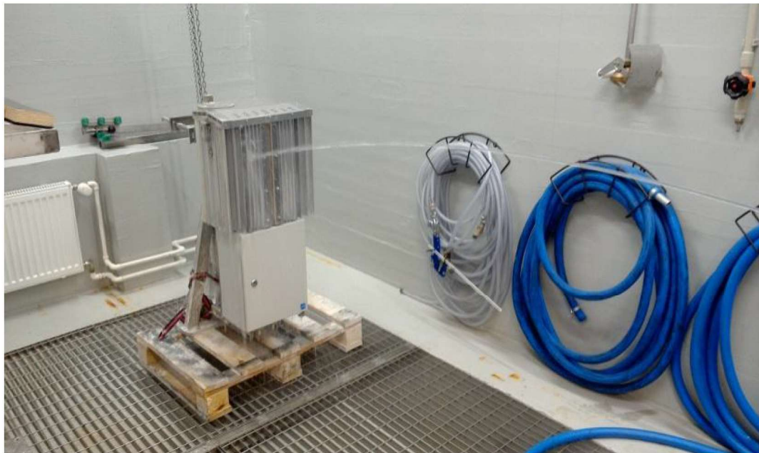
Photograph 2. The test setup for water test.
