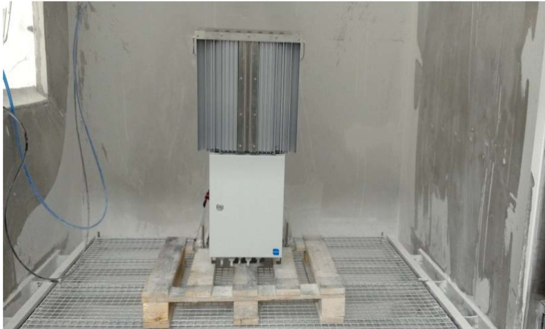
Photograph 1. The test setup for dust test.
