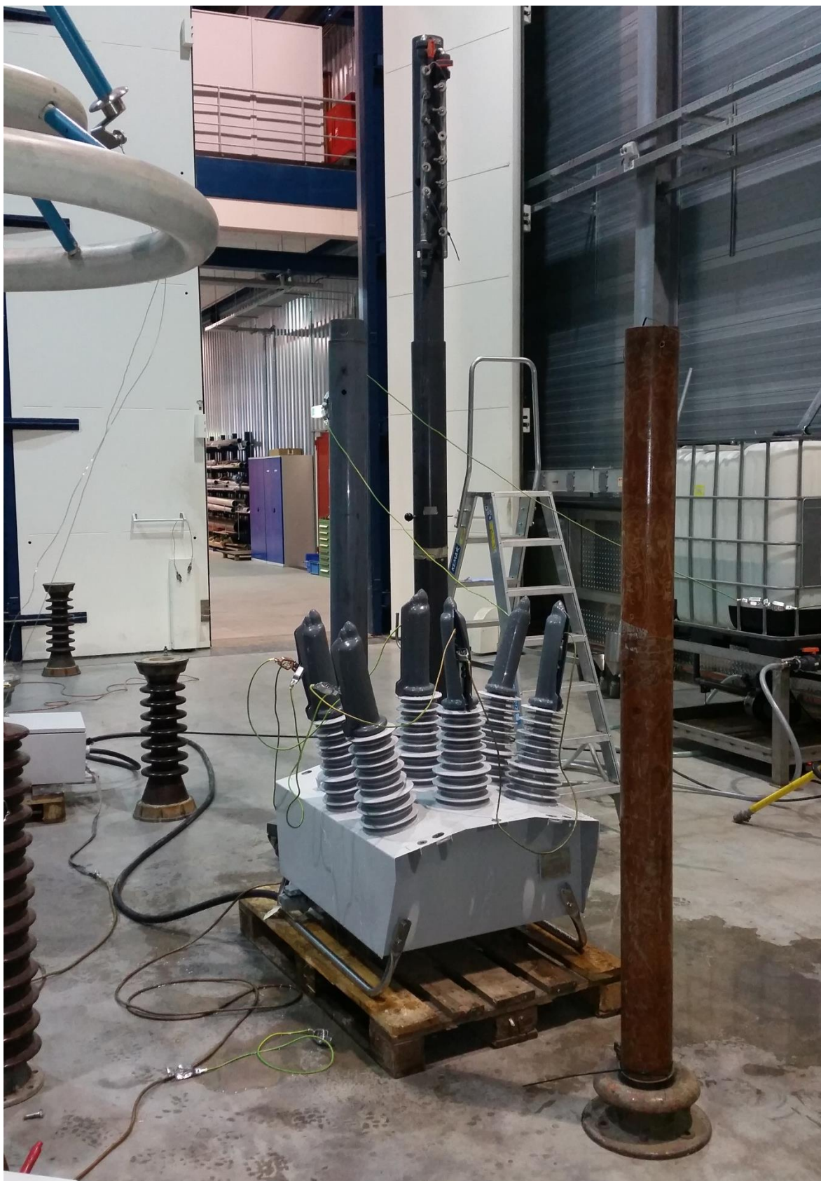
Test setup for the wet power-frequency voltage tests.
