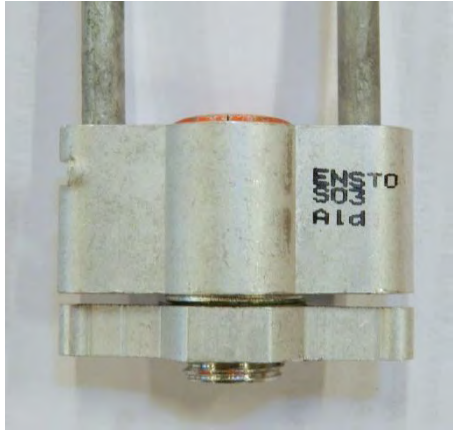
Picture 3: Markings on the clamp's body
