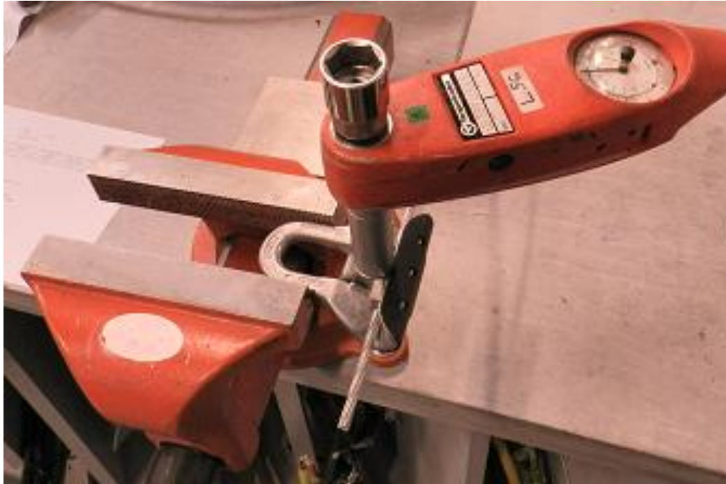
Picture 2: Bolt tightening test set up.
