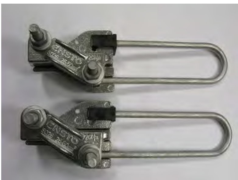
Picture 3: Samples after UV-test
