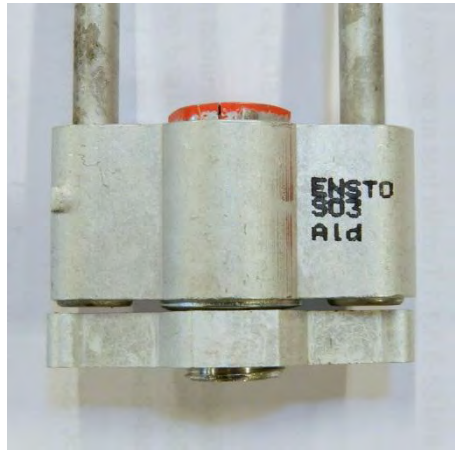
Picture 3: Markings on the clamp's body
