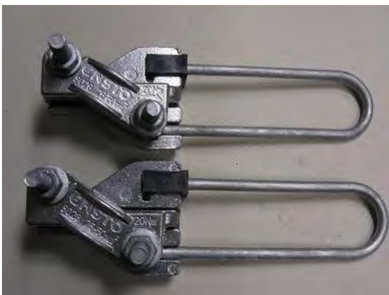
Picture 2: Samples before UV-test
