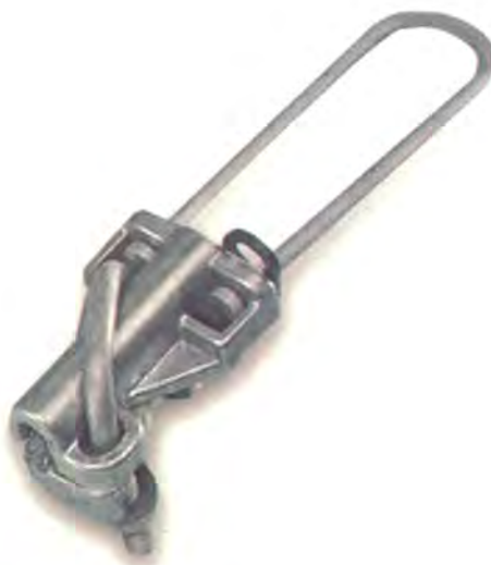
Picture 1: Tested tension clamp SO28
