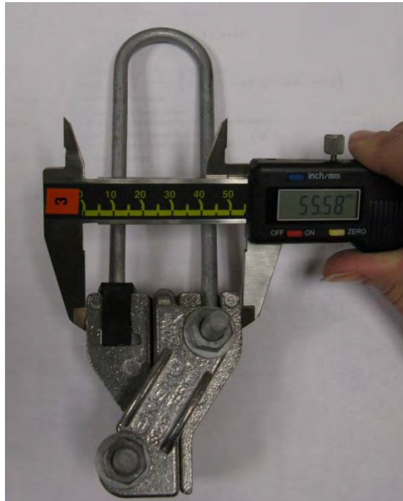
Picture 3: Clamp under the dimensional test
