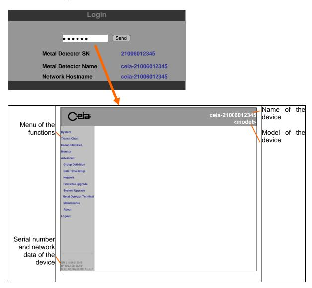
NOTE: In case of repeated error messages, stating that a wrong password has been entered, verify, in local programming, whether the baud rate setting of the device is 57600 (BR parameter).
