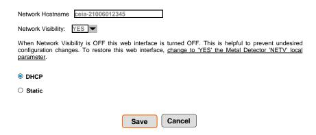
If static addresses are used, click on *Static* and enter the network data. Press *Save* to confirm. A new setting of the IP address is automatically updated as *Save* button is pressed and the page is redirected to the login box. If the hostname has been modified, a system reboot must be carried out: wait until the reboot phase is completed, then access the unit again by entering the new IP address in the URL field.
